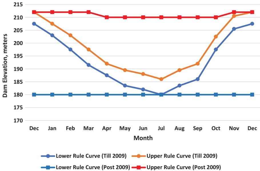
**Figure 2.** Operating rule curves. Adapted from MWSS (2014a, 2014b). Above the lower rule curve, all water allocations are met. Below the lower rule curve, urban water supply is prioritized over irrigation requirements.
